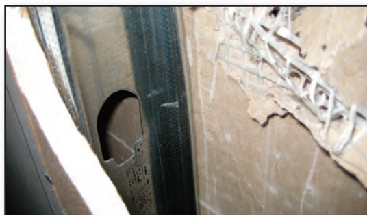
Soft body impact test using ViperStud.
