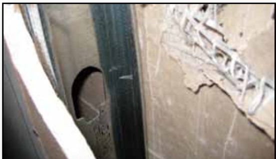
Soft body impact test using ViperStud.
