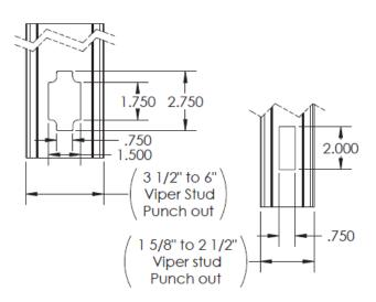
Figure 3 - CEMCO's Knockouts
